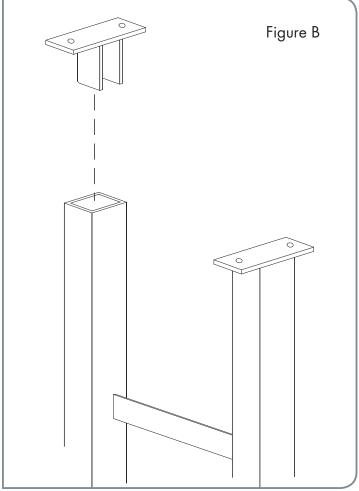
cut to fit your ceiling height (factor in 1/8" for thickness of the second Hidden Base Plate when cutting).
