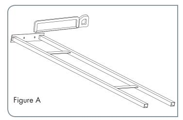
1. Cut off first welded mounting plate: On one section of the Wall Series Frame only, squarely cut the posts flush with the mounting plate to remove it (Figure A). Clean off any resulting burrs with a metal file. This will leave one section with a mounting plate and another open ended.
