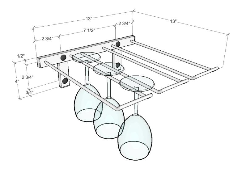
Note: A minimum of 1 inch above the rack and 12 inches down from the top of the rack are recommended clearances, but may vary by the height of the stemware stored.
