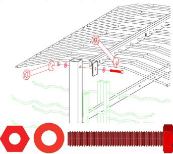
5. Finishing steps – Fully tighten all screws (especially Crossrail Assembly Screws) and snap mounting hole covers in place. Fill with  $^{\alpha}$
