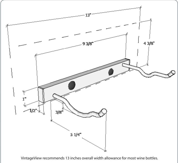
Mounting holes and overall demisions are identical for Left and Right options.
