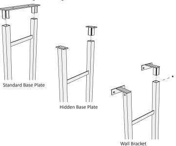
6. Install the frame - Position the assembled frame, ensuring it is plumb both front to back and side to side, using a level and fasten at the top through all available mounting holes. Fasten the extension brackets to the wall and then secure the bottom of the frame through the mounting holes in the mounting plates.
