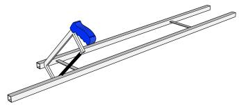
3. Assemble the lower frame - Insert the C-channel of the extension brackets into the end of one frame section and ensure that they fully seated, with the horizontal plate flush against the end of the frame. Install the bottom mounting plate option into the opposite end of the frame by sliding the C-channel into the frame as shown below and securing with a self-drilling screw through the side of the frame.
